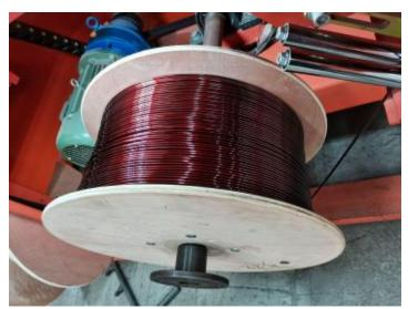
Coils winding. Once is ended the wire enameling, the wire is assemblied in particular spools to be later on weighed and sold.
